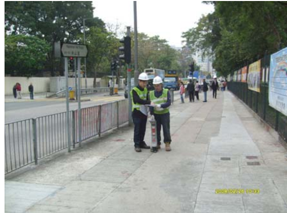
Photo 1: Field Measurement of Coating Defect Survey
